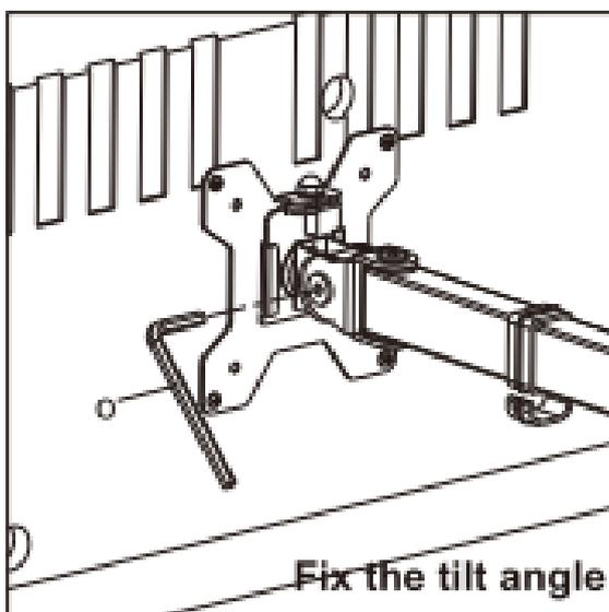
Tighten the bolt with the supplied Allen Key(o) to fix the tilt angle.
