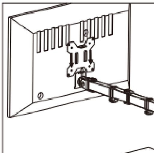
Slide the monitor onto the head of Swivel Arm(d) as shown in the above diagram.
