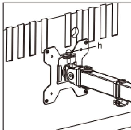
Install the security Nut(h). Make sure the security nut is installed before you rotate the monitor.
