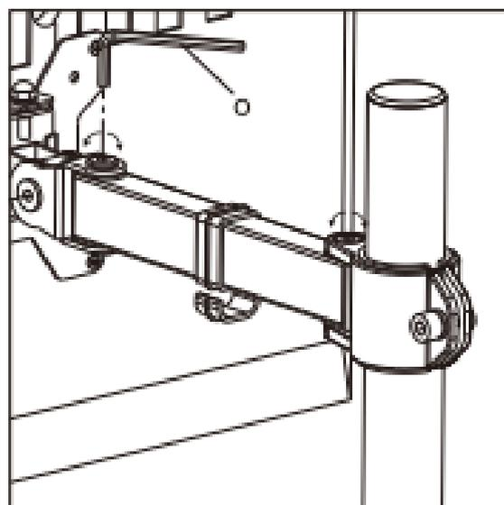
Use the supplied Allen Key(o) to make the necessary adjustments.
