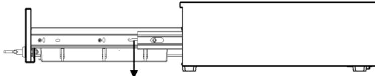
Press down the locking handle of slide on right hand side
