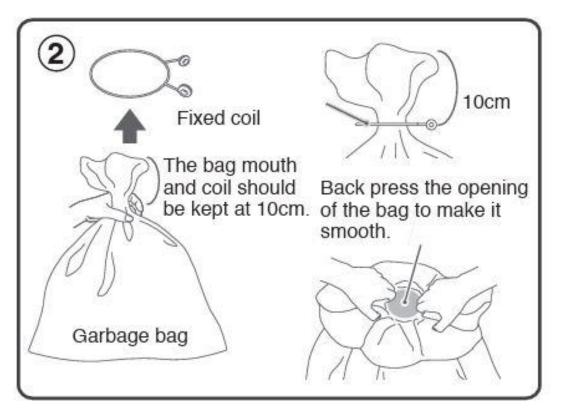
Fill the bag with air and hold it with your hand at the top. Then put the clamp on the top of the bag and open the inlet of the bag again so that the clamp is at a height of 10 cm.
