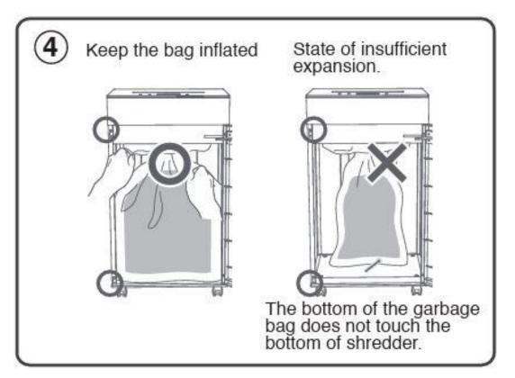
The trash bag should contain air and touch the bottom of the shredder.
