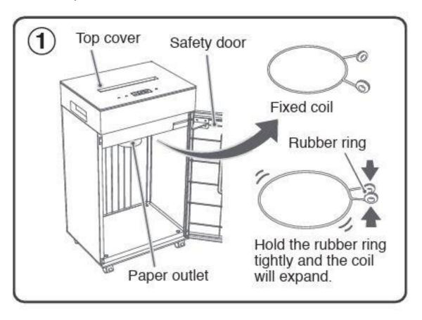
Underneath the top cover, there is a handle in the lower left corner. With it, open the security door to the right and the paper outlet will be closed. Then remove the clamp located on the paper hole.
