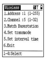
PDT-8B and wireless base station must be matched, the paired principle is: 1 wireless base station supports multiple PDT-8B at the same time, but address cannot be same for one base station, one base station uses one different channel value.
