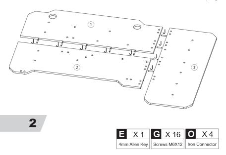
Note: The horizontal bar on the Iron Connector should be perpendicular to the seam of the table panel splice
