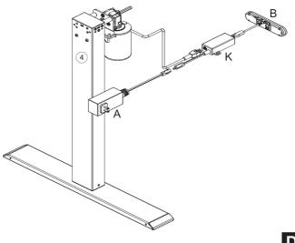
Use D -Wire Clips to tidy up the wires.
