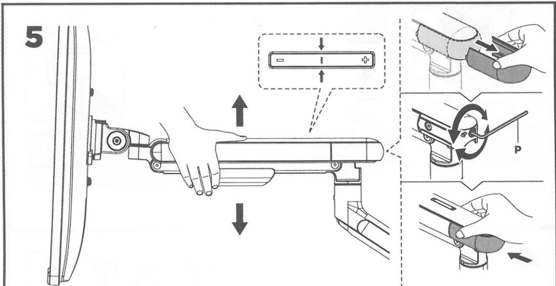
To properly balance the arm with monitors mounted, adjust the spring tension using the supplied Allen Key as follows:
