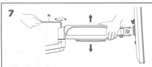
To properly balance the arm with monitor mounted, adjust the spring tension using the supplied Allen Key as follows:
