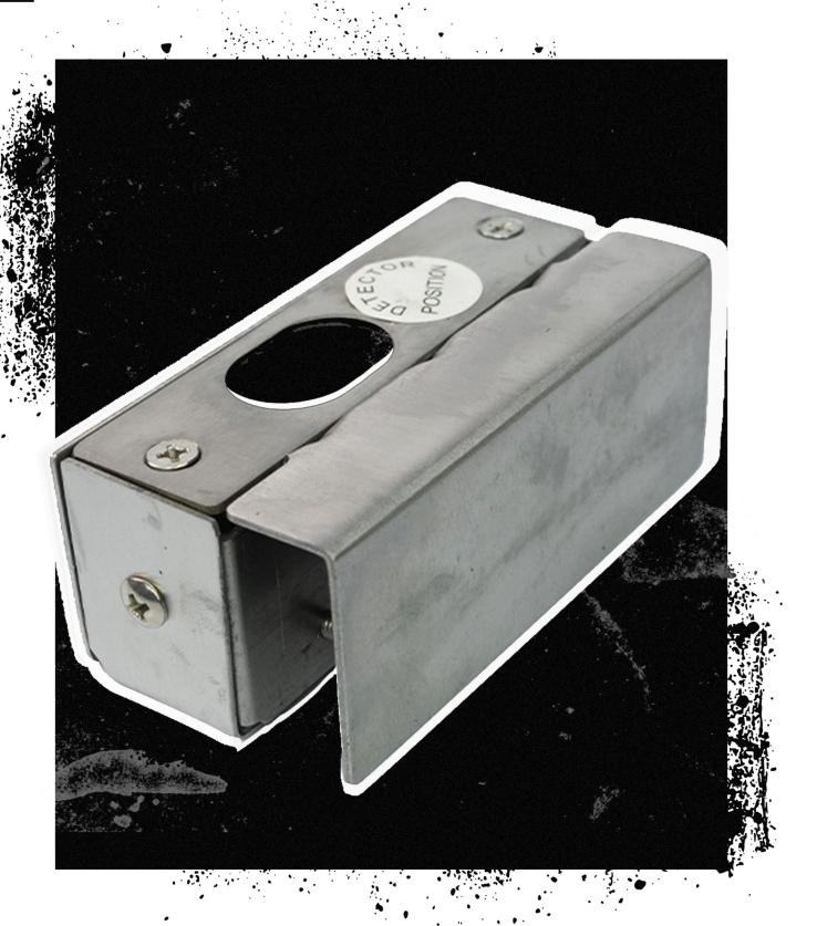
SecureEntry-SC20 is an abutment designed to work with electronic surface lock. Designed to be applied to glass doors. Allows you to lock the door. It is equipped with a position detector that works with the electromagnet, allowing the bolt to be extended at the appropriate moment and thus closing the door.
