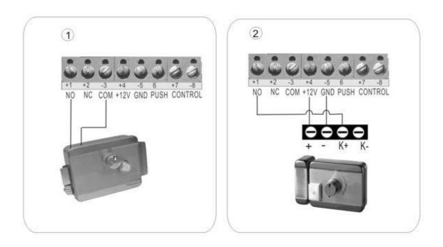
**Remark!** The electronically controlled interlock must be switched to 0 seconds delay to prevent the electric interlock from burning out.
