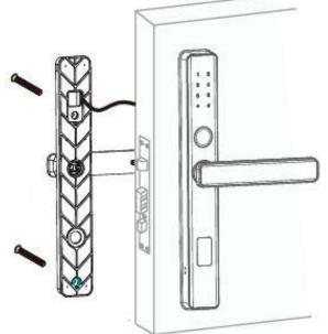
Place the screws into the corresponding holes, fix the back panel and tighten the screws, install the battery and close the battery cover.
