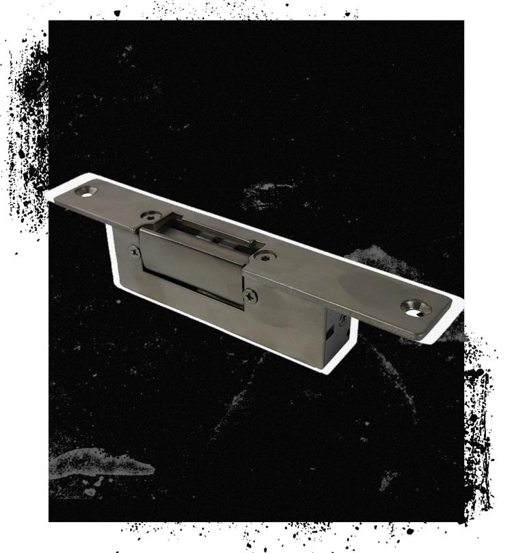
SecureEntry-ES200 is a rugged and sturdy stainless-steel electric striker designed for mortise locks. Safety is ensured by the power of the hitch with a lifting capacity of 500 kg. The device supports DC12Vi voltage and 200 mA current. The electric striker needs a constant flow of power to unlock the door.
