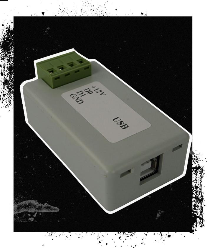
SecureEntry-ConWG-USB is a converter designed to support access control devices. Allows you to connect devices equipped with Wiegand 26 or 34 interface to a computer using the included USB cable. It supports 9-12V and works with most popular operating systems.
