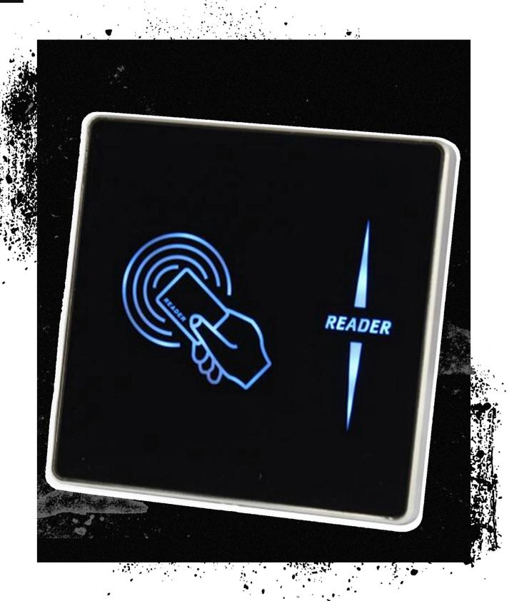
SecureEntry-CR60LF is an RFID card reader offering control and management of access to buildings and premises. It supports 125 kHz cards. Features compact shape and elegant design. It offers a DC voltage of 9-16V and has a Wiegand 26 interface with the ability to change to Wiegand 34.
