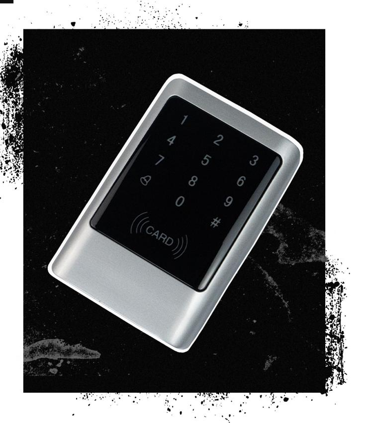
SecureEntry-AC900LF is a standalone access controller. Offers authentication by RFID card and individual password. It is equipped with Wiegand 26 interface, which gives the possibility to connect with external devices. It features DC12V and operates at 125 kHz.
