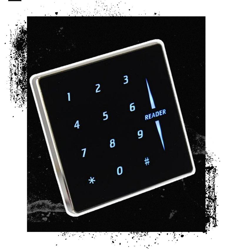
SecureEntry-AC800LF is a sleek RFID card and password reader offering building and room access control and management. It supports 125 kHz cards. Features compact shape and modern design. It offers a DC voltage of 9-16V and has a Wiegand 26 interface with the ability to change to Wiegand 34.
