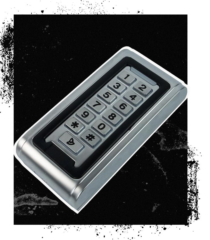
SecureEntry-AC500 is a numerical access keypad, used to control access to buildings and premises. Supports 125 kHz frequency and DC12V voltage. It is made of strong alloy zinc and offers an IP65 rating for protection against water ingress. Allows you to unlock the door with a password and RFID card
