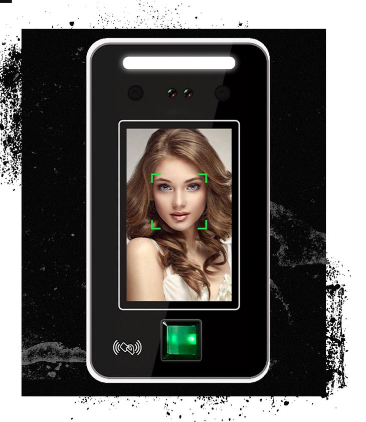
SecureEntry-AC300 is an advanced device used to control the Access with facial recognition. Access to rooms and recording of working time is additionally possible by means of Fingerprint, password and RFID card.
