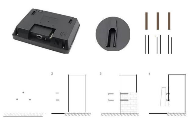
1.Make three marks on the wall where the mounting holes are drilled
