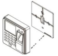
3. Align the holes drilled in the wall and screw the back cover to the wall with Screws
