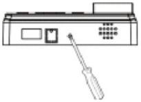
2. Remove the back cover from the device
