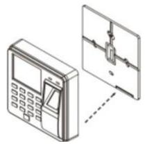
5. Lock the back cover with the bottom screw
