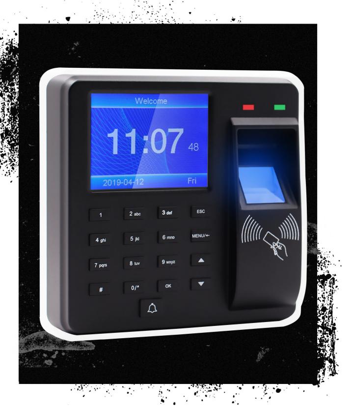
**The CTR10 model** is an advanced multifunctional device, which is used to control and manage access to posz individual rooms and buildings, as well as to record the attendance of employees in the enterprise.
