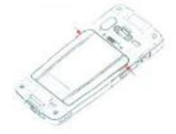
**4.** Open the battery cover and remove the battery in the direction indicated
